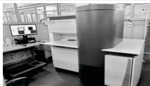
X-ray photoelectron spectroscopy (XPS) Make: K-Alpha Company: Thermo Fisher Scientific
