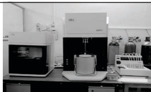
Surface Area Measurement Facility (BET) Model: BELLSORP MAX II & BELCAT-II Company: MicrotracBEL Corp
