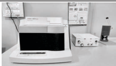
Differential Scanning Calorimetry (DSC) Model: DSC-60 Plus Company: M/s Shimadzu (Asia Pacific) Pte Ltd
