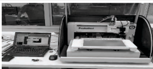
PCB Prototyping Machine (PCB) Model: LPKF-PCBProtoMat S103 Company: LPKF Laser & Electronics AG
