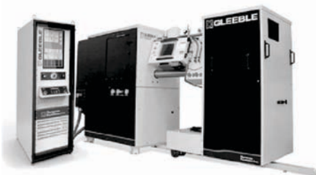
Thermal mechanical Physical Simulator and Testing Equipment Company: Dynamic System Inc. Model: Gleeble -3800 - GTC
