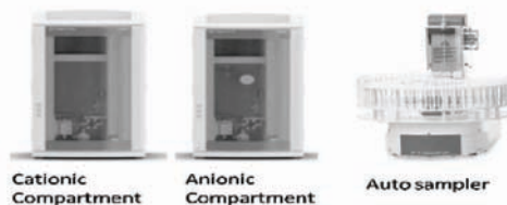
Ion – Chromatography (IC) Model: Dual channel 930 Compact IC Flex ChS/PP --- Metrohm Company: Metrohm AG
