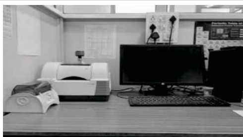
Fourier Transform Infrared Spectroscopy (FTIR) Model: Nicolet iS5 Company: THERMO Electron Scientific Instruments LLC
